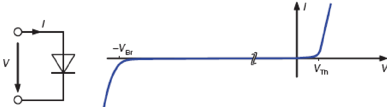
Figure 3.18 Symbol and I/V characteristic curve of a p-n diode: in the forward direction the diode only conducts from the threshold voltage V_{Th} , in reverse direction, there are high currents in the case of exceeding the breakthrough voltage V_{Br}
