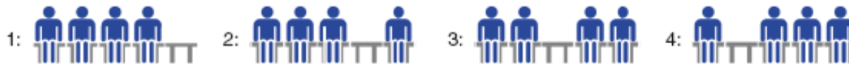
Figure 3.10 Transport of current by means of holes. The electrons move to the right one after the other. Therefore there is a “hole movement” in the opposite direction. The situation is comparable to the movement of people along a row of seats
